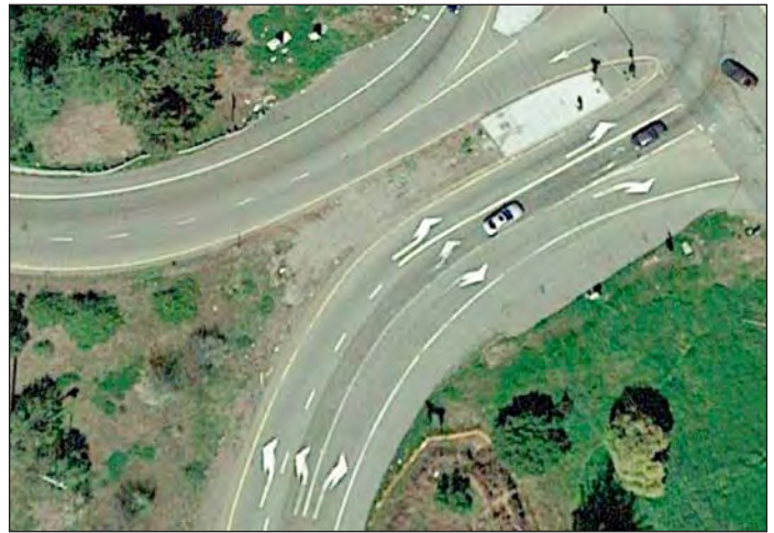
Increasing the capacity of off-ramp terminal with local roadway.
