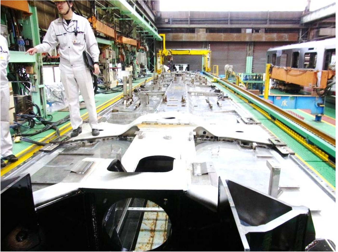
Car No. 115 bolster, connecting the body to the truck, at bottom of underframe.
