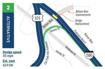
Drivers would exit US 101 northbound between the top of Cal Park Hill and the Bellam Boulevard off-ramp. The connector would be an elevated structure that crosses Andersen Drive and follows the alignment of Simms Street before merging with I-580 eastbound.
