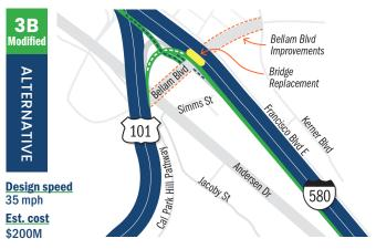
Drivers would exit US 101 northbound on a separate lane near Bellam Boulevard and merge onto I-580. The off-ramp from eastbound I-580 to Bellam Boulevard would be replaced with a new, separated off-ramp.
