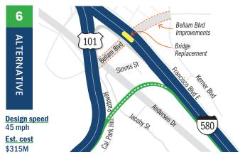
Drivers would exit US 101 northbound between the top of Cal Park Hill and the Bellam Boulevard off-ramp. The connector would be an elevated structure that crosses over Jacoby Street, Andersen Drive, and the Golden Gate Bridge Highway & Transportation District bus yard before merging with I-580 eastbound.
