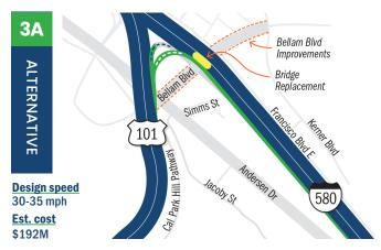
Drivers would exit US 101 northbound near Bellam Boulevard and merge onto I-580 eastbound on a connector that crosses over the existing off-ramp.
